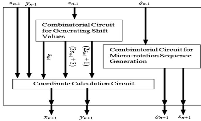
Fig. 5. Block diagram for the stage.
