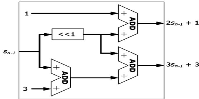
Fig. 6. Combinatorial circuit for generating the shift values.
