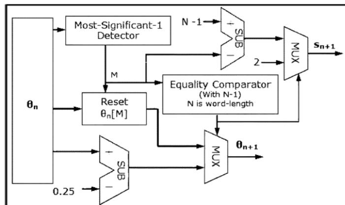
Fig 7. Micro-rotation sequence generation.
