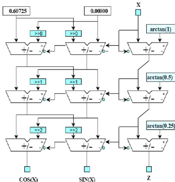
Fig.2. Parallel/Cascaded CORDIC
