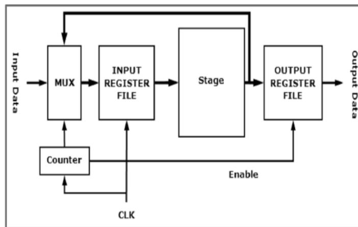
Fig.4. Recursive architecture of the proposed CORDIC processor.
