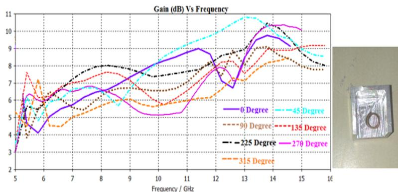
Fig. 4 Gain plot for U-wall configuration at various helix rotation angles
