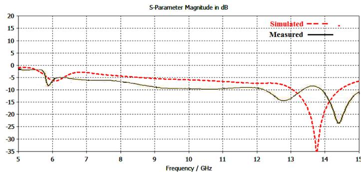
Fig. 6 Plot of reflection coefficient at 270° helix rotation
