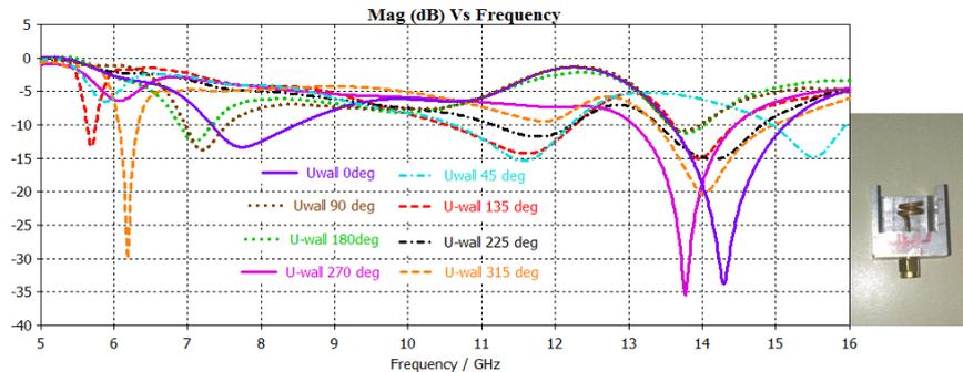
Fig. 3 Comparative plot of reflection coefficient at various rotation angles
