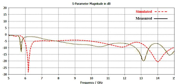
Fig. 7 Plot of reflection coefficient at 315° helix rotation
