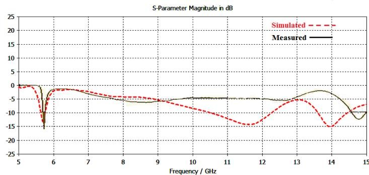
Fig. 5 Plot of reflection coefficient at 135° helix rotation
