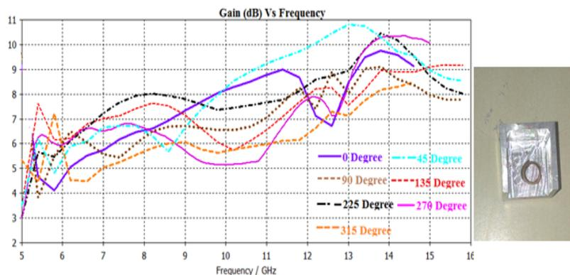
Fig. 4 Gain plot for U-wall configuration at various helix rotation angles
