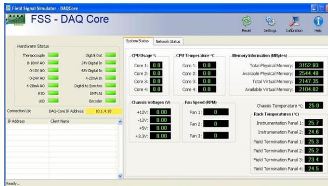
FIGURE 4: DAQ CORE – Snapshot for System Status for Server
