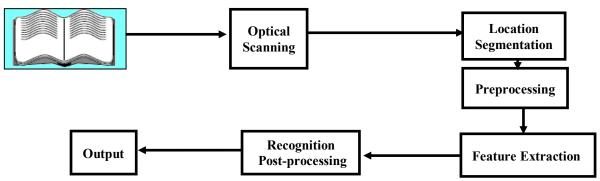
Fig.- 2: Components of typical OCR/ODR system
