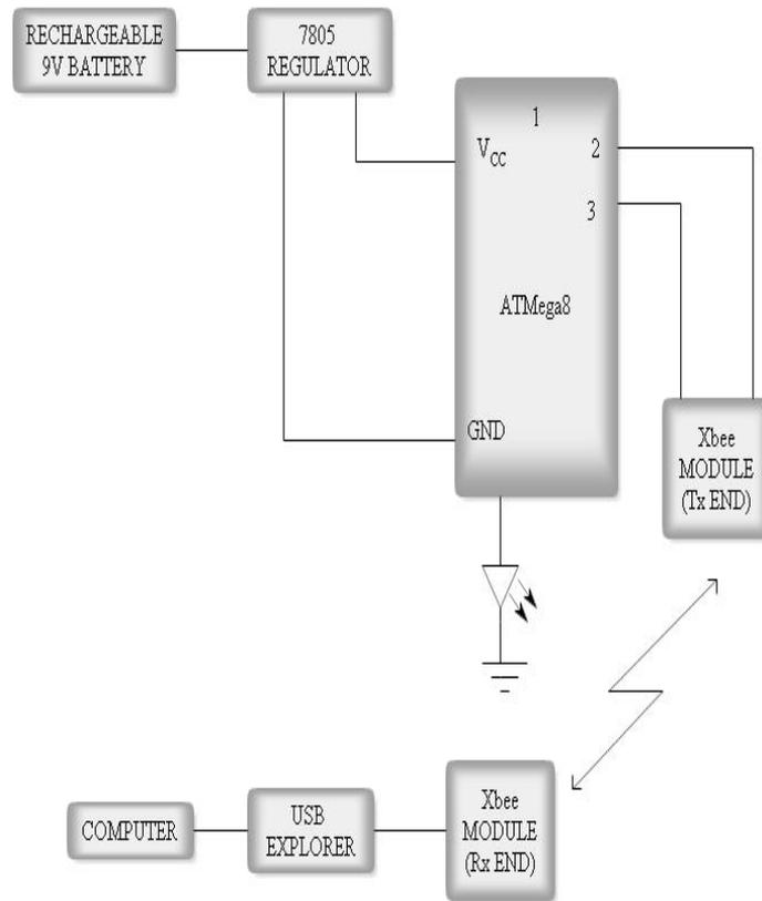
Fig 1: Block Diagram
