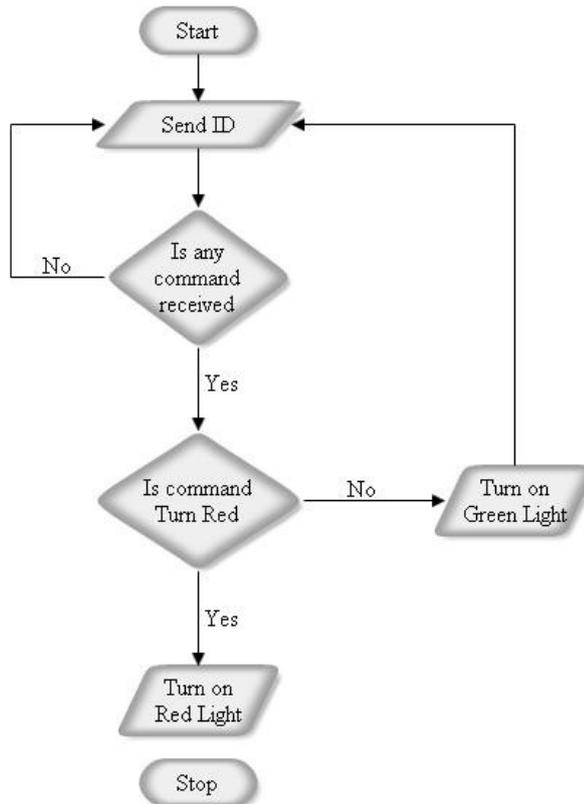
Fig 3: Flow Chart for the Electronic Ticket
