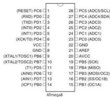
Fig 4: Pin Diagram of ATmega8 Microcontroller
