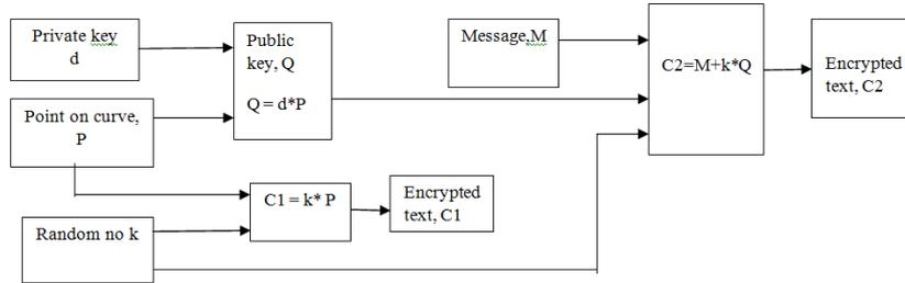
Figure 1.2 – Encryption at sender site
