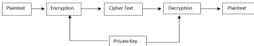
Figure 1.1 – Encryption/ Decryption Process
