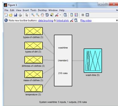
Fig: 2 Fuzzy Logic Controller for Wash Time
