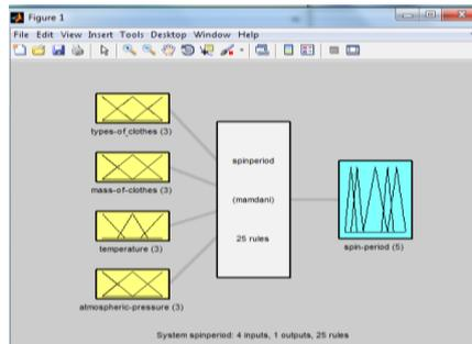
Fig: 9 Fuzzy Logic Controller for Spin period
