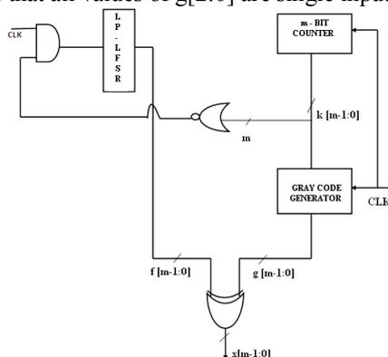
Figure 3. Low Power Test Pattern Generator
