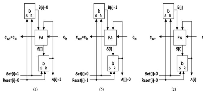
Fig. 2. Configurations of the accumulator cell of Fig. 1.
