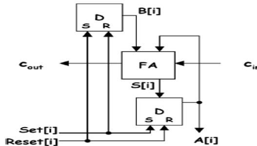
Fig. 1. Accumulator cell.
