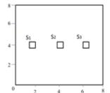
Figure4. Sensor node deployed on ceiling at 3 meter height within room.
