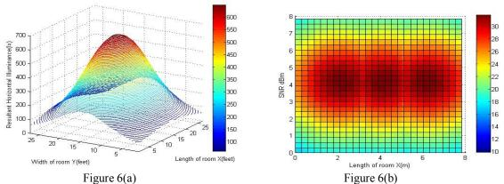
Figure 6(a). Resultant horizontal illuminance of all three WSN node. Figure 6(b) Shows SNR distribution of three sensor nodes.
