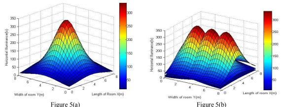
Figure 5(a) Figure 5(b) Figure 5(b) shows Horizontal illuminance(lx) of single WSN node and Figure 5(b) shows Horizontal illuminance of each node among three WSN node.
