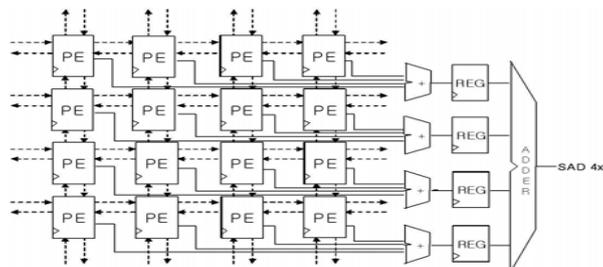
**Figure 9 PE Array 4x4 architecture**
