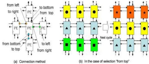
Figure 12 PE Configuration
