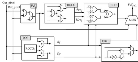
Figure 4 block diagram of the self-detection/correction operations
