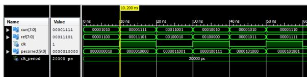
corrected processing element output
