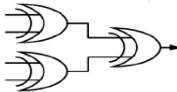
**Figure 8 Error detection circuit.**
