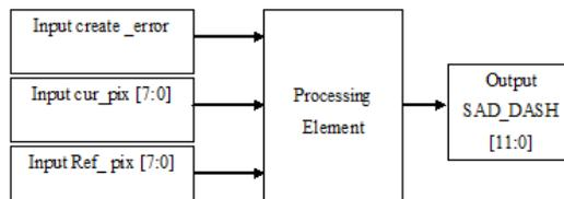
Figure 5 Processing Element Module Schematic Diagram
