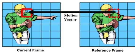
Figure 3 Block Matching between Current & reference frames
