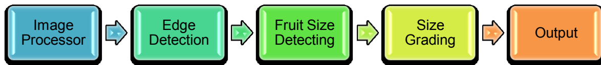
Figure 3: Fruit image size detecting and grading flow
