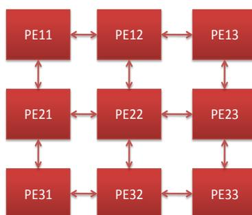
The network of processing elements consists of nine PEs and all are internally connected to each other. PE11 is connected to PE12 and PE21, PE12 is connected to PE11, PE13 and PE22, PE13 is connected to PE12 and PE23. Similarly other PEs are connected to its neighbour PEs. The PE22 is connected to four processing elements those are PE12, PE21, PE23 and PE32.
