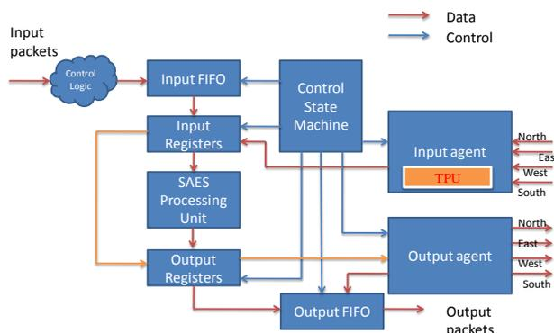
Accepting packets into FIFO for processing. Data packet is accepted if the temperature of the core is less than the specified threshold temperature. Here the threshold temperature is set to 90. Input FIFO is required because input data can come at a rate different from the processing speed. Hence it should be buffered in the FIFO.
