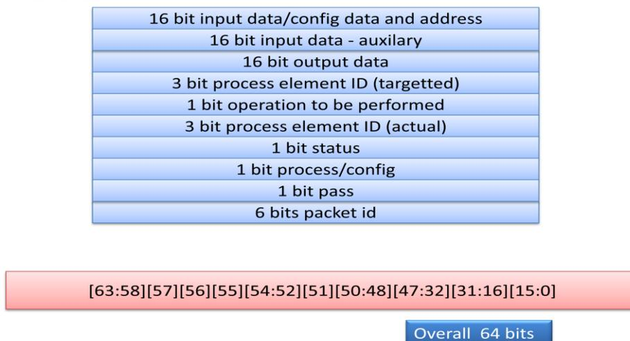
The above figure shows the packet format, each packet consists of 64 bits which is divided into ten sections. A task is encapsulated as a packet. Task in this project is to encrypt or decrypt data.
