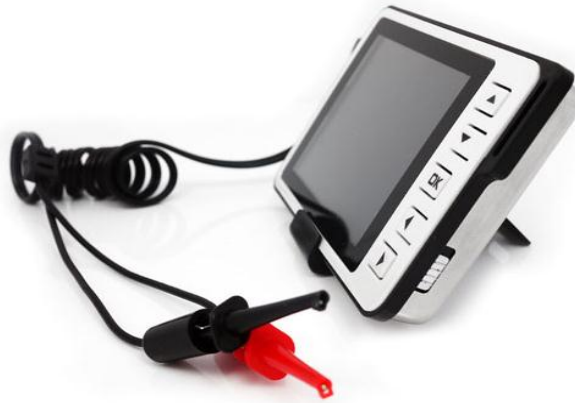
Fig. 1 : Handheld All-in-One Electronics Lab Assistant Device with USB Connectivity
