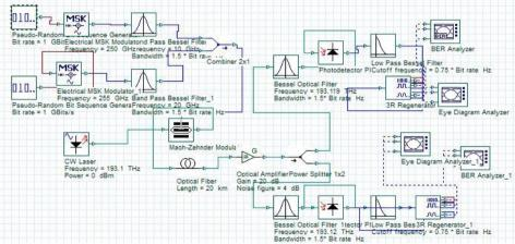
Figure3(c)RoF system using MSK technique
