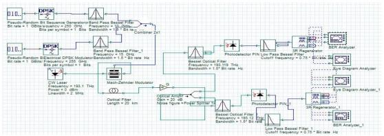
Figure 3(a)RoF system using DPSK technique
