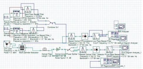
Figure3(d)RoF system using CPFSK technique
