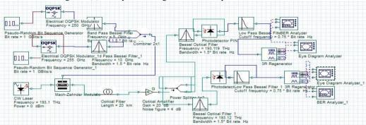
Figure 3(b)RoF system using OQPSK technique
