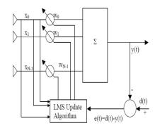
Fig.7: LMS Adaptive Beam Forming Network
