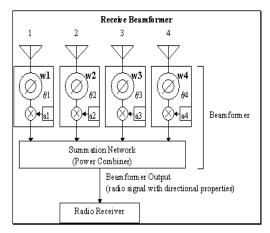
Fig.4: receiver beam former
