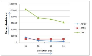
Figure1: Number of packets sent for AODV, DSDV and ZRP for different scenarios
