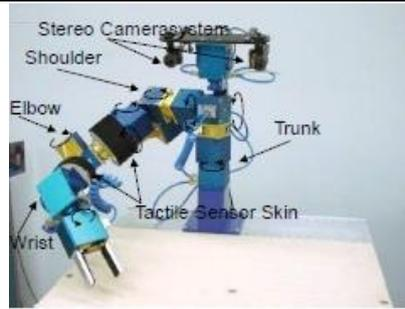
Figure 1: The service- and assistance robot CORA. A seven DoF manipulator arm is mounted on a one DoF trunk which is fixed on a table. The robot possesses a two DoF stereo camera head with microphones.
