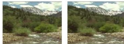
Fig. 16. Super-resolution result of an image with rich texture regions. Left: bicubic interpolation, and right: our approach.
