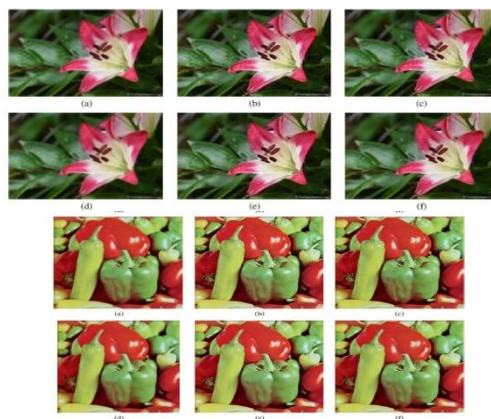
Fig. 13. Super-resolution results of offline images "Lily" and "Peppers": (a) Directional interpolation, (b) backprojection, (c) learning-based pair matching, (d) directional interpolation after adaptive regularization, (e) backprojection after adaptive regularization, and (f) learning-based pair matching after adaptive regularization.
