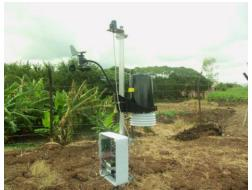
Figure 3.1 Integrate sensor suite at field
