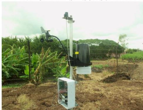
Figure 3.1 Integrate sensor suite at field
