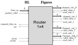
Figure 1: Block Diagram of Five Port Route
