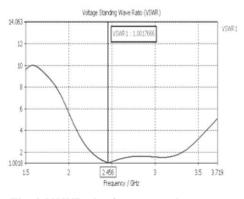
Fig. 3 VSWR plot for proposed antenna
