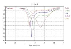
Fig. 5 Return loss plot for various values of G
