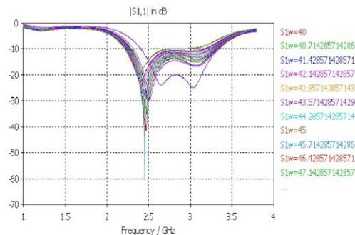
Fig. 7 Return loss plot for various values of  $S_w$ .
