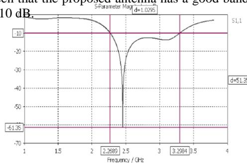
Fig. 2 return loss plot of proposed antenna
