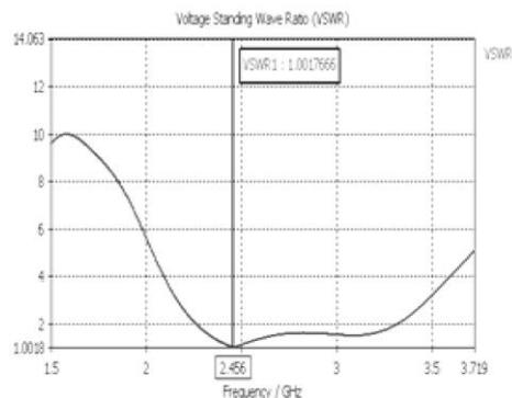
Fig. 3 VSWR plot for proposed antenna
