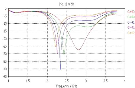
Fig. 5 Return loss plot for various values of  $G$
