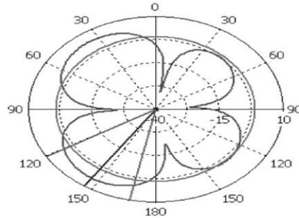
Fig.4 Radiation pattern plot for proposed antenna
