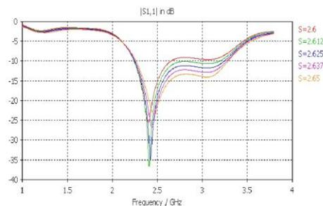
Fig. 6 return loss plot for various values of  $S$
