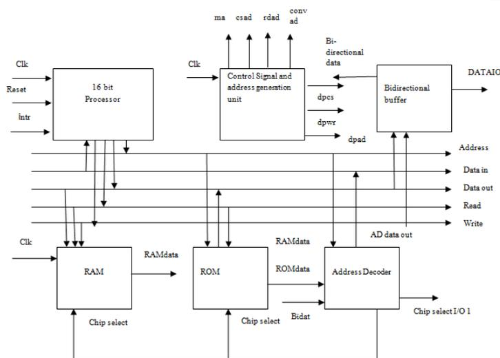
Figure 4: Block diagram of the developed FPGA
