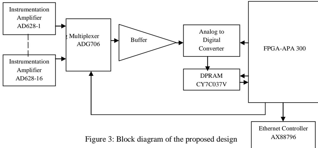
Figure 3: Block diagram of the proposed design
