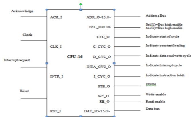
Figure 5: Top view of the 16 bit processor
