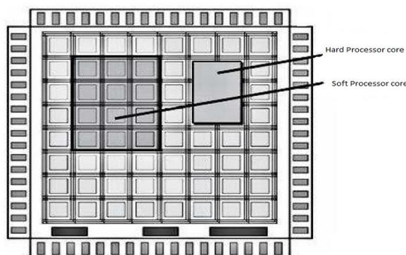
Figure 2: An example of FPGA hard and soft processor.
