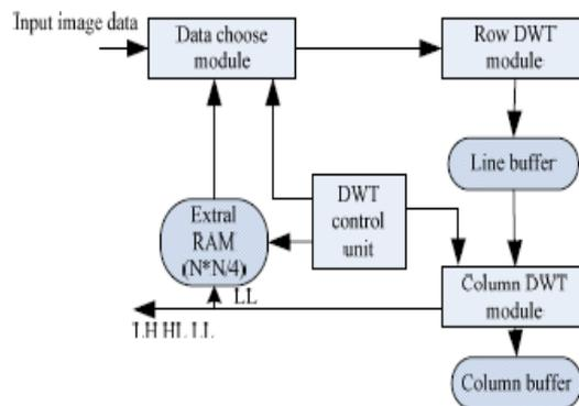
**Fig 4. Proposed 2-D DWT architecture**
