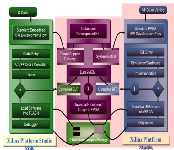
Fig 8. Embedded Development Kit Design Flow
