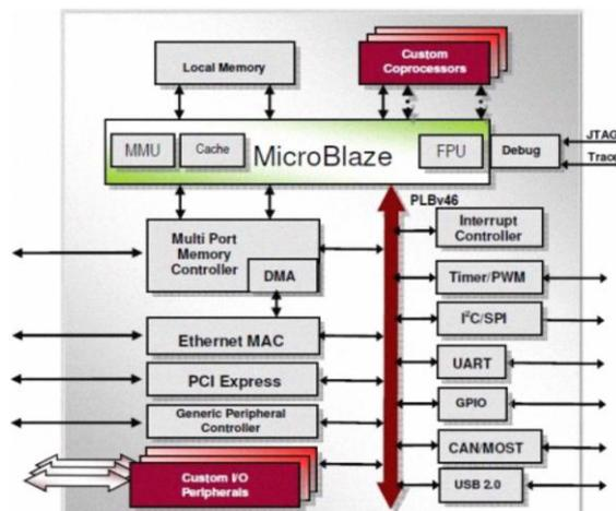
**Fig 7. Microblaze Architecture Block Diagram**
