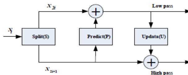
Fig 6. Block diagram of the lifting scheme.
