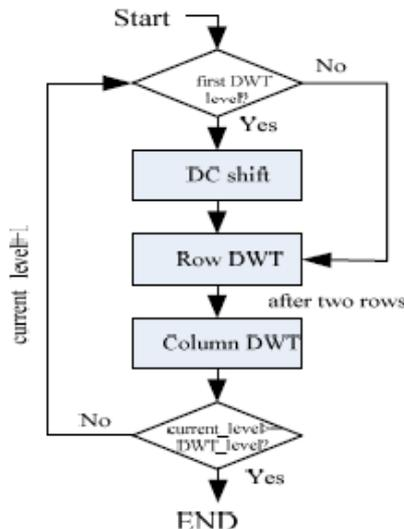
**Fig5. FSM of DWT control unit**
