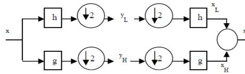
Fig 2. DWT analysis and synthesis system
