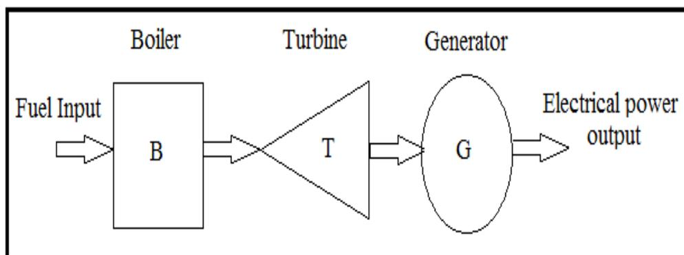
Fig.1 Simple model of thermal generation system
