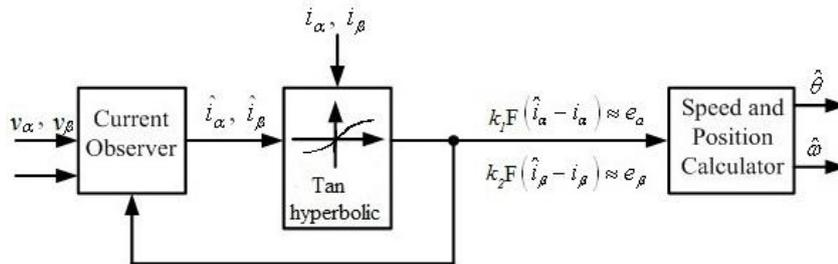
Fig. 3 Sliding Mode Observer with Tan Hyperbolic Function
