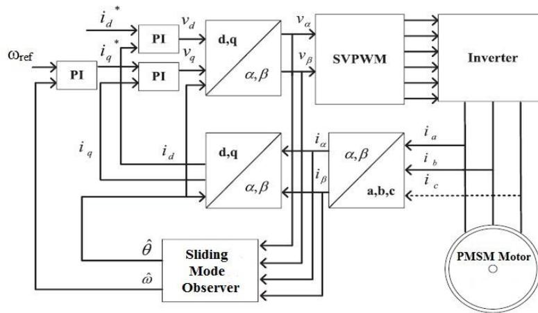
Fig.1 Overall control structure of PMSM
