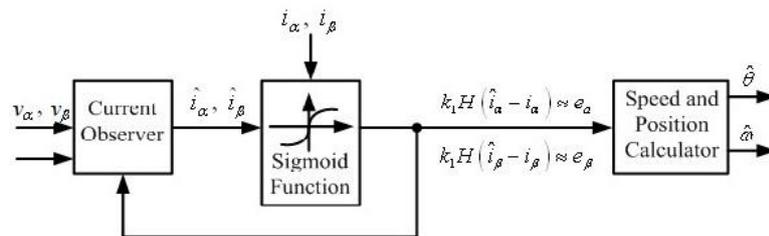
Fig.2 Sliding Mode Observer with Sigmoidal function
