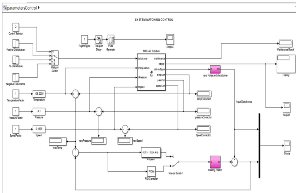
Fig. 6. Simulink Diagram for the Online-Inspection System (Feature Matching Model).
