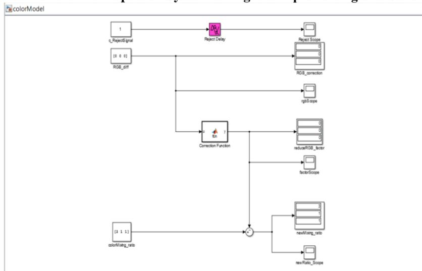
Fig. 5. Simulink Diagram for the Pre-Inspection System (Colour Model).
