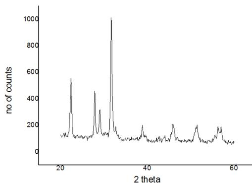
Fig 2. XRD of BFO thin film grown on PtSi.
