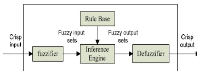
Fig.3.General architecture of fuzzy logic system (FLS)
