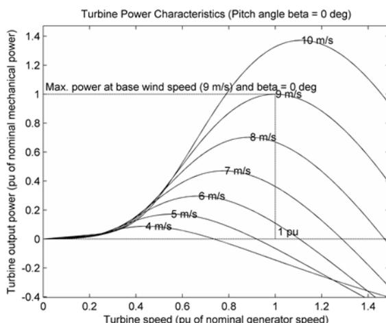
Fig.2.PowerCharacteristics of Wind Turbine
