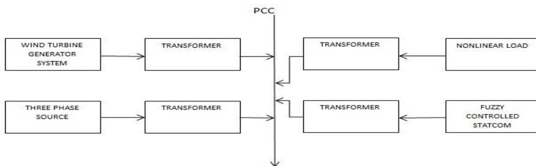
Fig.1.Simulated windfarm Topology
