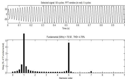
Fig.6.FFT of source current without STATCOM
