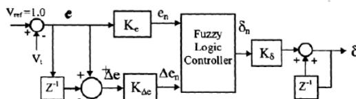
Fig.4. Control circuit for STATCOM
