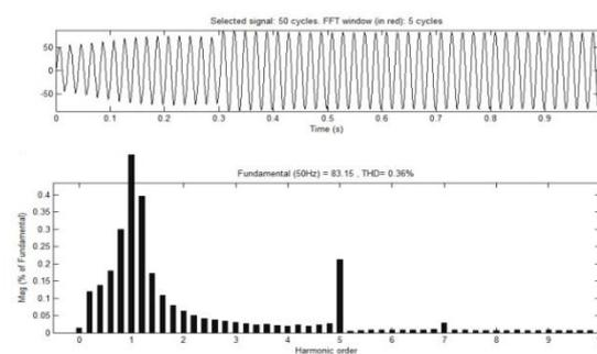
Fig.7.FFT of source current with STATCOM
