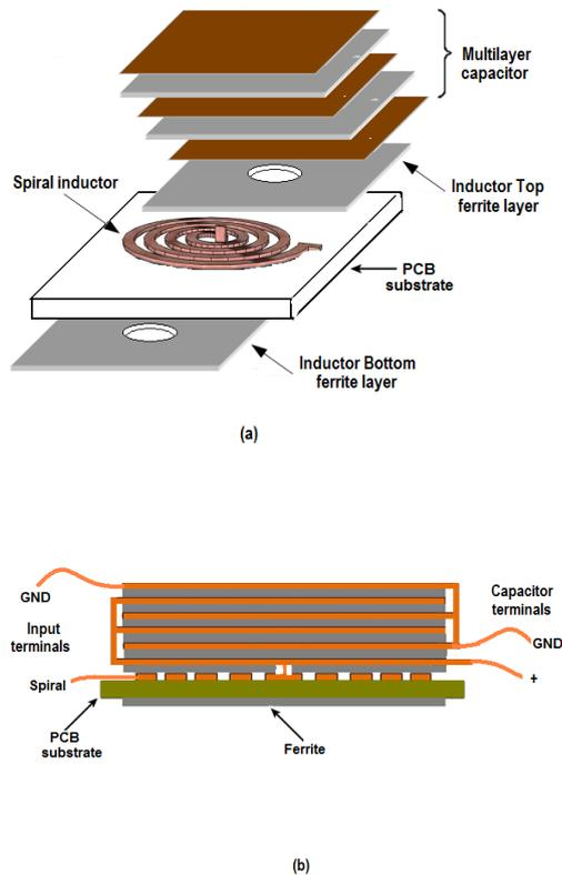
Fig. 1 - Exploded (a) and cross section (b) views of the structure
