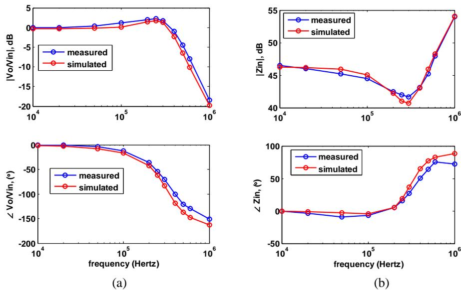
**Fig. 10** - Measured and simulated Frequency response of Output to input ratio  $V_{out}/V_{in}$  (a) and Input impedance (b) of the integrated structure
