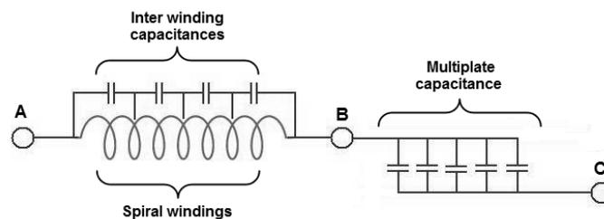
Fig. 2 - The equivalent circuit model of the structure
