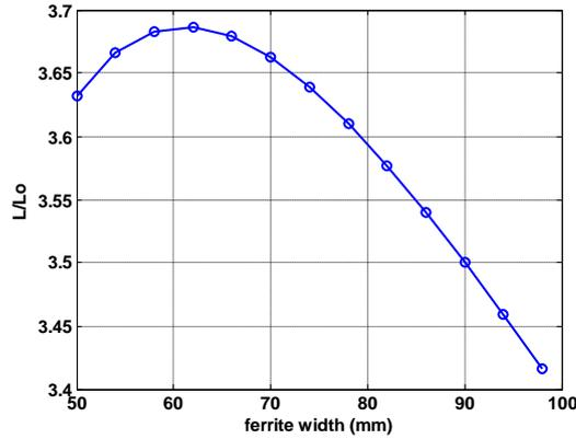
Fig. 4 - Magnetic factor  $K_m$  when  $D_o$  varies from 48 mm to 98 mm
