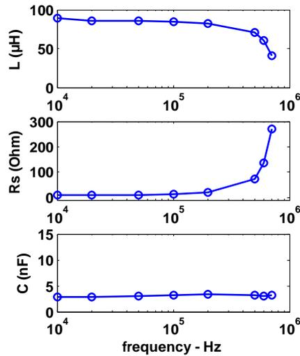
Fig. 9 - Frequency characteristic of inductance, series resistance and capacitance
