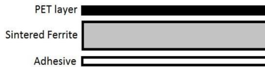
Fig. 5 - Flexible ferrite sheet presentation [6]
