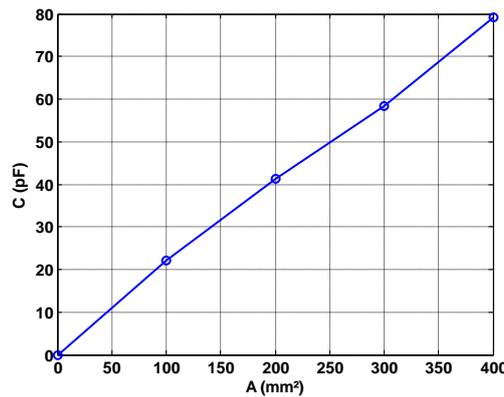
Fig. 6 - Capacitance variation with surface area
