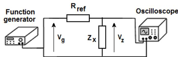
**Fig. 8 - Inductance and capacitance measurement setup**
