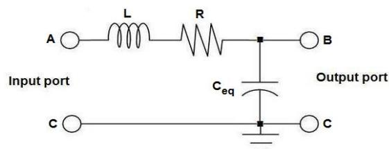
Fig. 3 - Equivalent circuit of the structure
