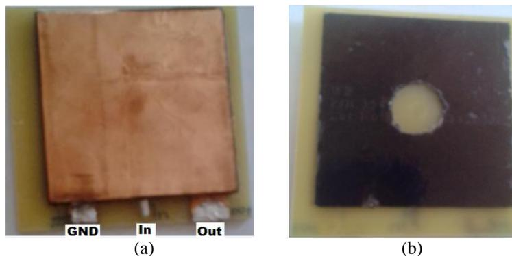
**Fig. 7** - Photograph of LC-filter: (a) – top side, (b) – bottom side
