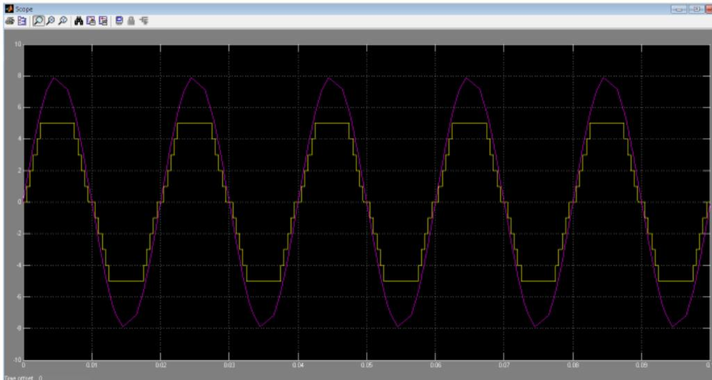
Fig. 5. Inverter voltages for a step in the amplitude of the reference current
