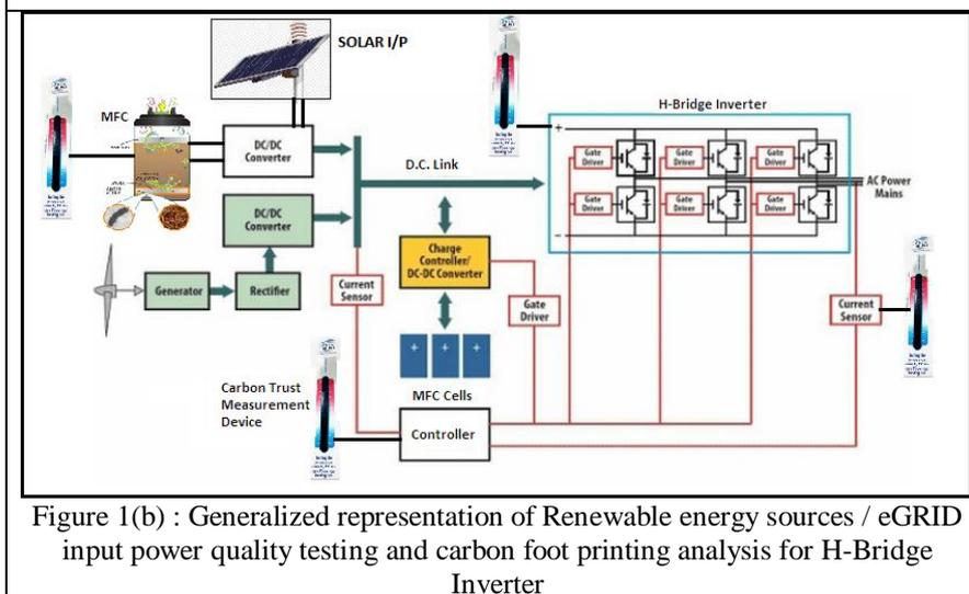
Figure 1(b) : Generalized representation of Renewable energy sources / eGRID input power quality testing and carbon foot printing analysis for H-Bridge Inverter
