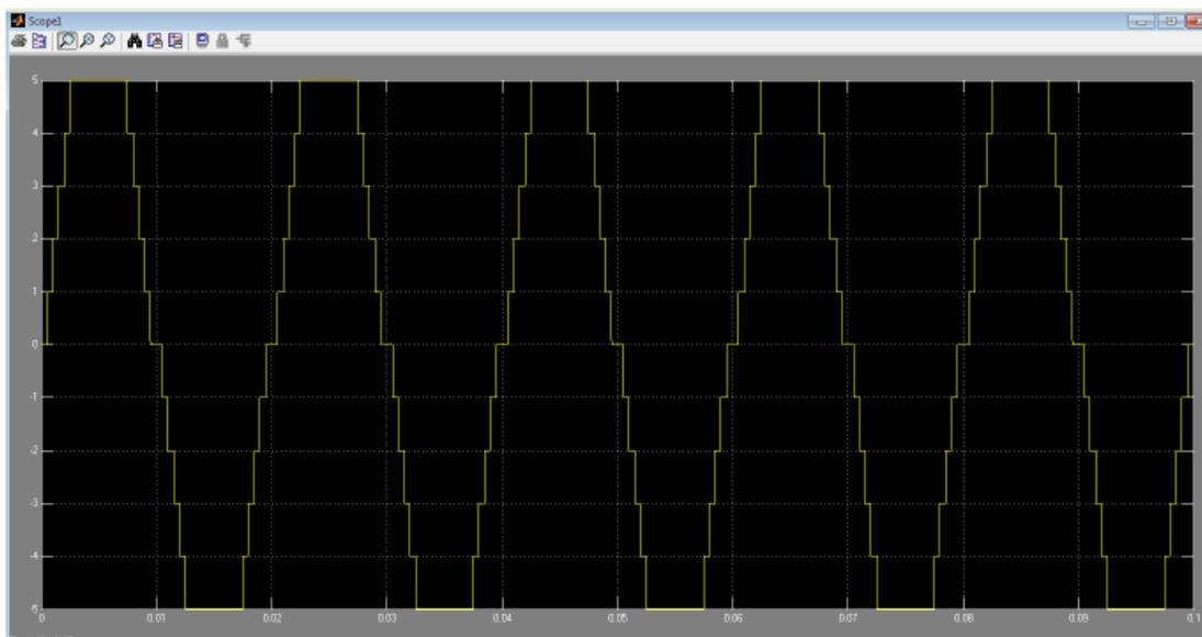
Figure 4. Load current in one phase for a step in the reference amplitude.
