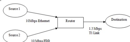
Fig1: Congestion in a packet switched network.
