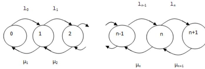
Fig 5: Poisson queues transition diagram.
