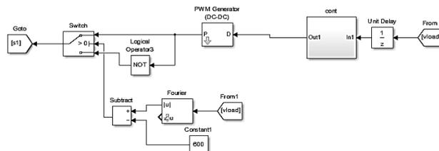
Fig. 5. Simulink model of a battery and boost converter control
