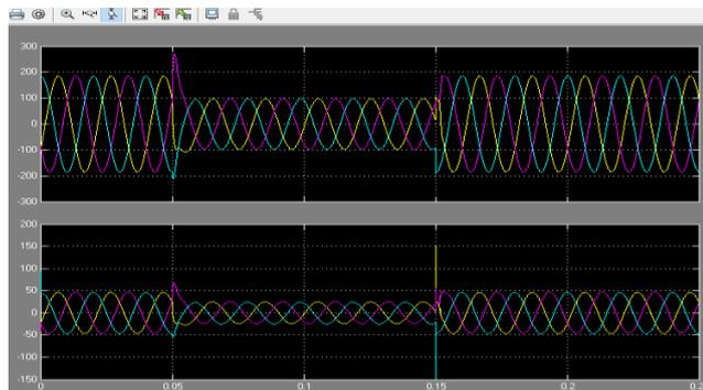
**Fig. .** Hybrid System Simulation results: Three phase sag to 50% of nominal voltage at load during faults in 0.05-0.15second
