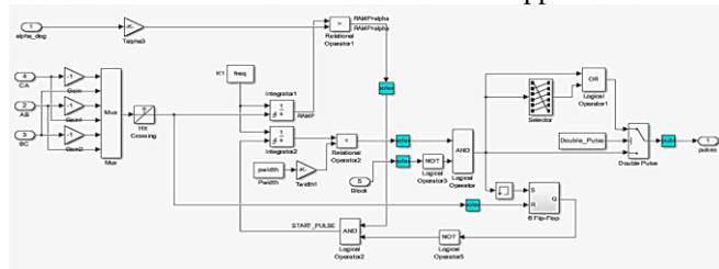
Fig. 7. Simulink model of DC-AC Inverter PWM Signal Generator
