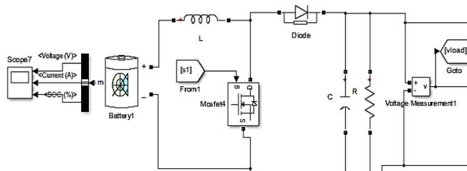
Fig. 4. Simulink model of a battery with DC-DC boost converter
