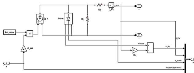
Fig. 3. Simulink model of a photovoltaic array
