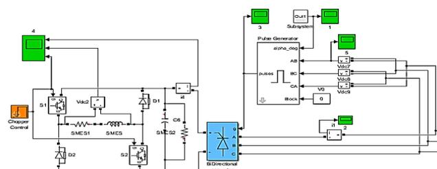
Fig. 6. Simulink model of SMES with DC-DC Chopper and DC-AC Inverter
