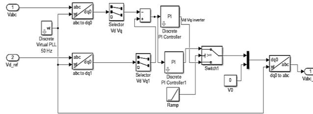
**Fig. 8.** Simulink model of PWM Signal Generator Controller
