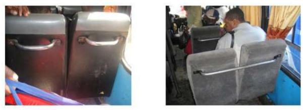
Figure 8 Unsafe structures in bus interior may hurt passengers or cause secondary impacts
