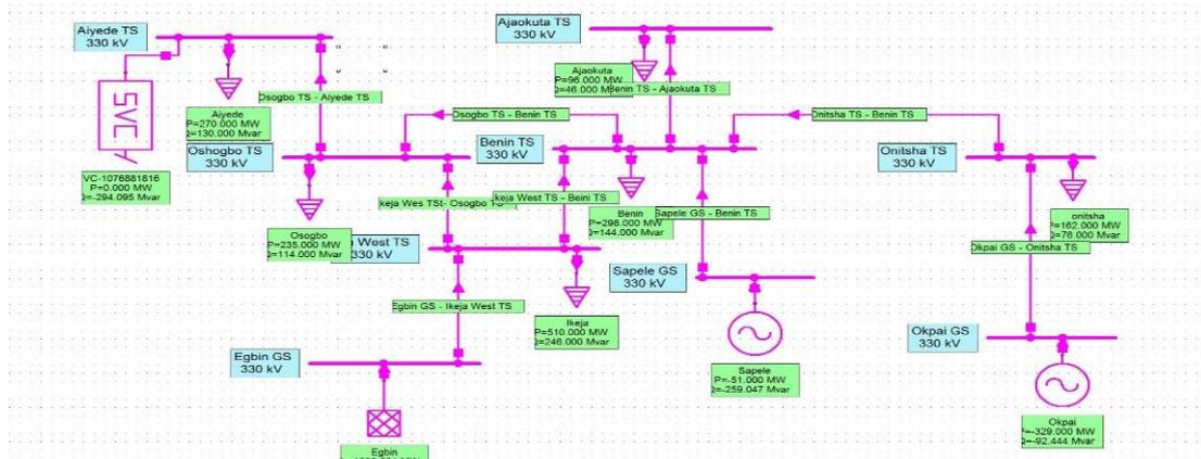
Figure no 3: The 330kV 9-bus Nigeria Power System with SVC
