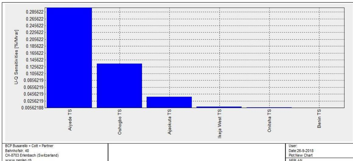
Figure no 5: Constant power static load V-Q sensitivities
