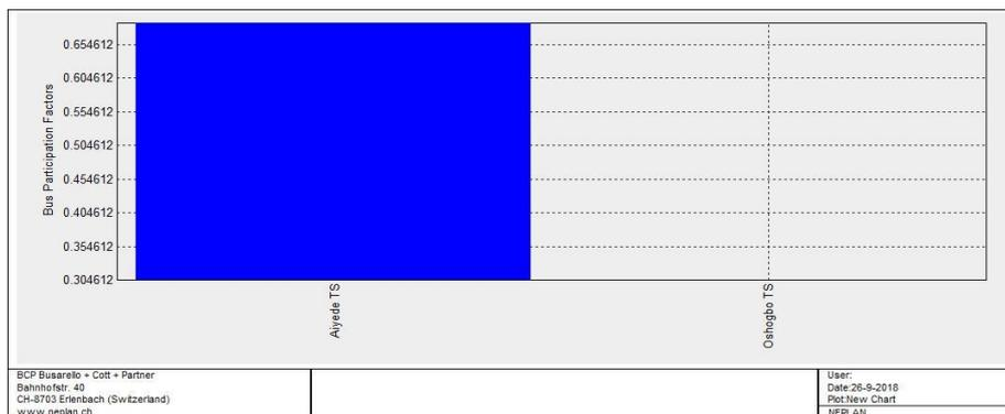
**Figure no 10:** Bus participation factor at the least eigenvalue of 7.7110 for constant impedance static load
