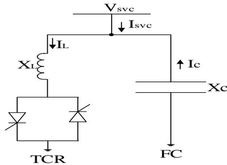
Figure no 1: Functional Diagram of a TCR-FC SVC<sup>14</sup>.
