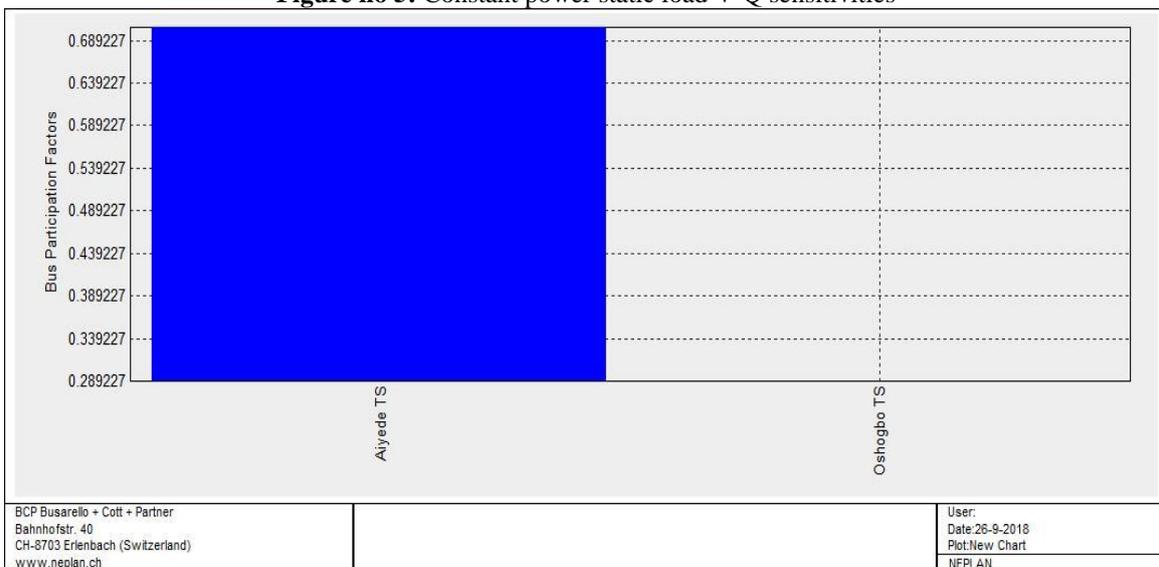
Figure no 6: Bus participation factor at the least eigenvalue of 2.4142 for constant current static load
