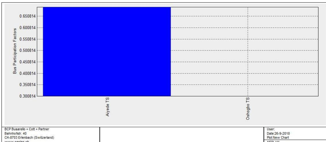
**Figure no 8:** Bus participation factor at the least eigenvalue of 6.4365 for constant current static load
