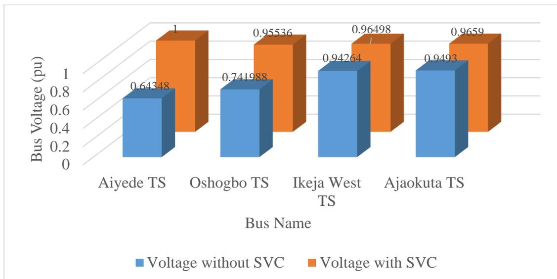
Figure no 4: Constant power static load weak bus voltage compensation representation
