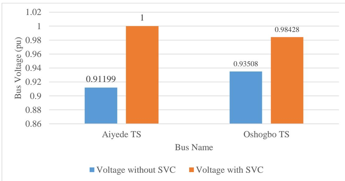
**Figure no 9:** Constant impedance static load weak bus voltage compensation representation
