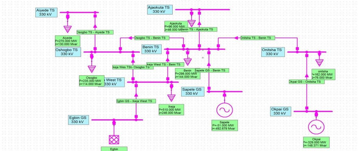
Figure no 2: The 330kV 9-bus Nigeria Power System without SVC
