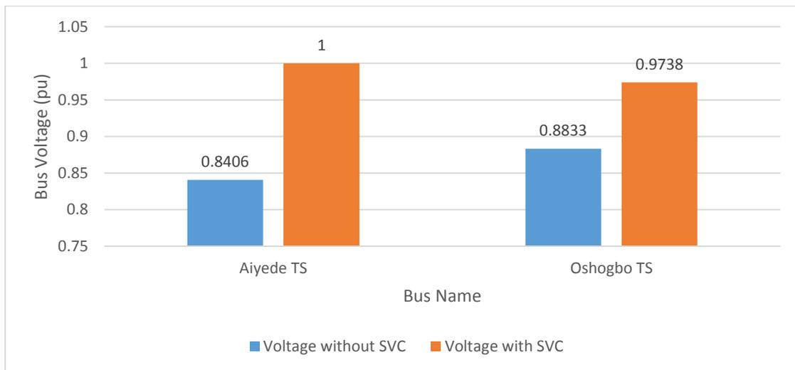
**Figure no 7:** Constant current static load weak bus voltage compensation representation
