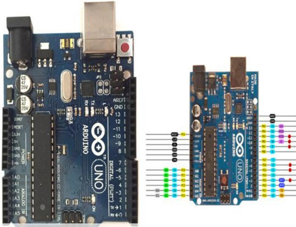
**Figure 2:** Arduino Microprocessor board and pin-out layout (source: Arduino UNO 2018)
