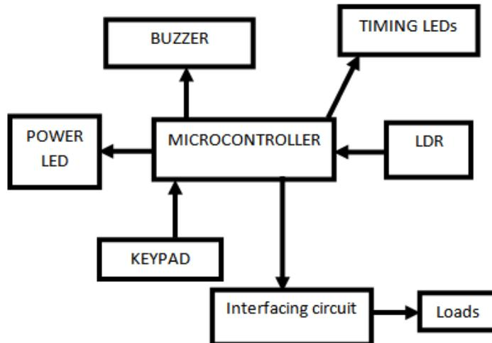
**Fig. 5:** System block diagram
