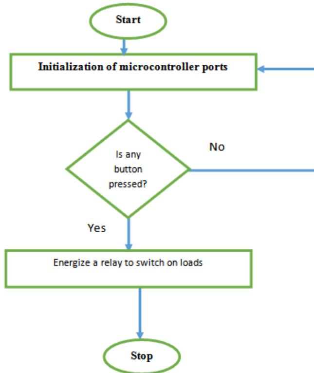
**Fig.6:** The system flowchart
