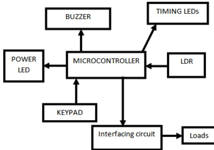
**Fig. 5:** System block diagram
