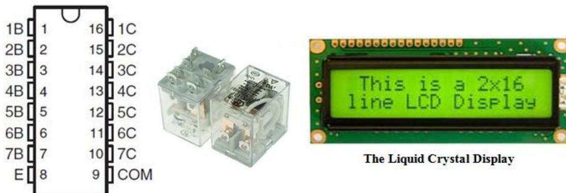
**Fig 4.** The ULN2003A Pinout, 12V Relay and LCD (source: futurelec.com)
