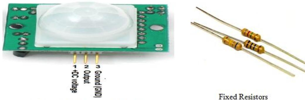
**Figure 3:** PIR sensor and fixed resistors.
