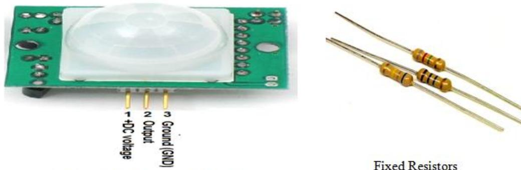
**Figure 3:** PIR sensor and fixed resistors.
