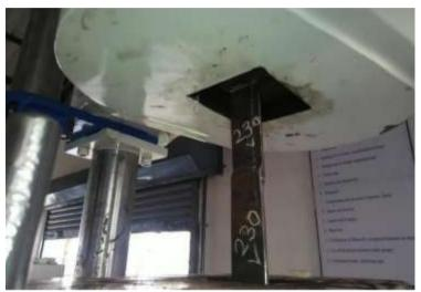
Figure 2 Sample specimen between the holding plates of the UTM during shear test.
