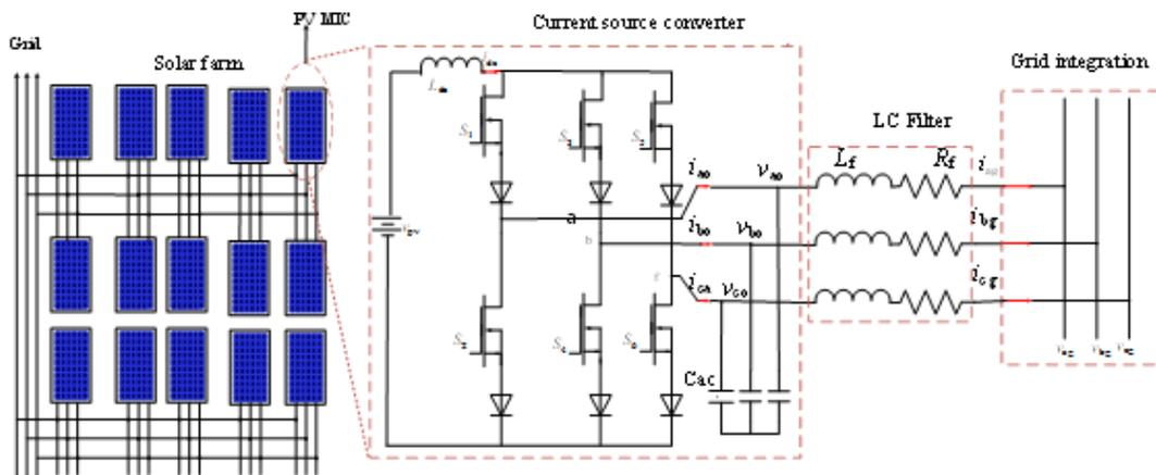
Fig.1. Block scheme for PV system
