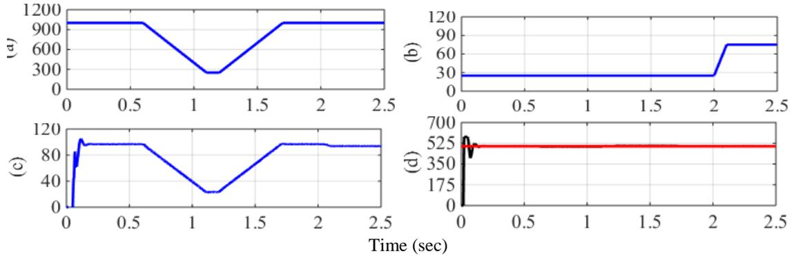
Fig.3, the dynamic response of PV based FLC-MPC (a) radiation signal (b) temperature signal (c) power
