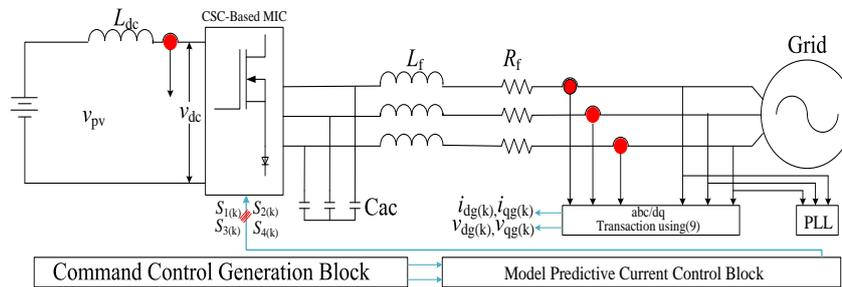
Fig.2. Block scheme for proposed control system
