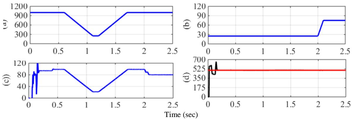
Fig.7, the dynamic response of PV based PI-PI (a) radiation signal (b) temperature signal (c) power response (d) DC voltage response
