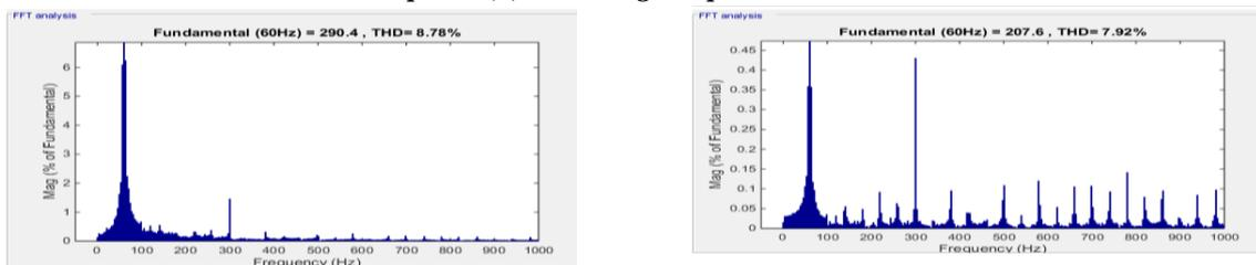
Fig.8. The THD of AC voltage and current based on PI-PI
