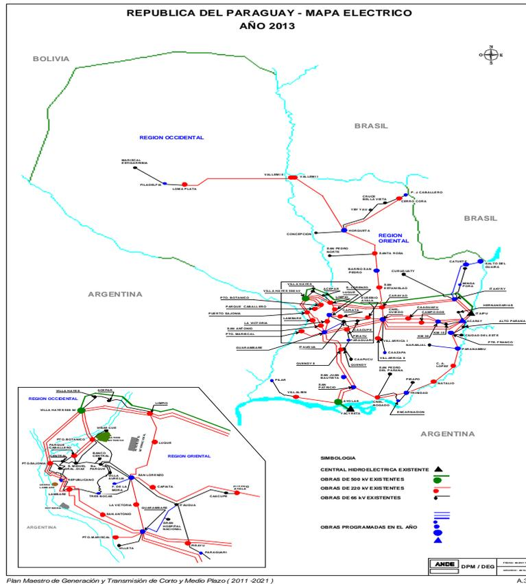
Figure 1. Master Plan of the Paraguayan Electric System. Source: ANDE (2013-2023)
