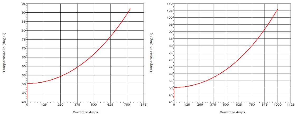
**Fig. 5** Comparison of Ampacities between ACSR Driver and ACCC type conductor under ambient temperature of 42°C. Source: Own and [8], 2018
