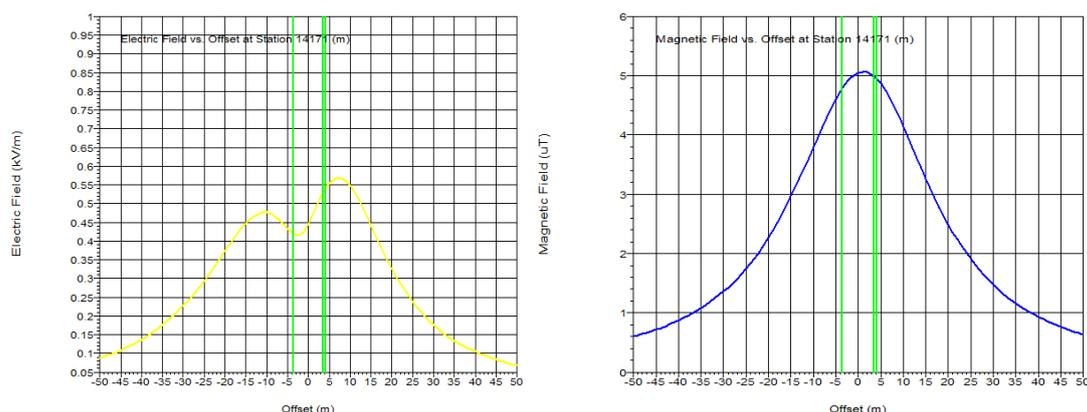
**Fig. 6:** Results of the evaluation of the electric field and magnetic field in the width of the easement strip of a 220kV transmission line with ACCC conductor. Source: [8], 2018
