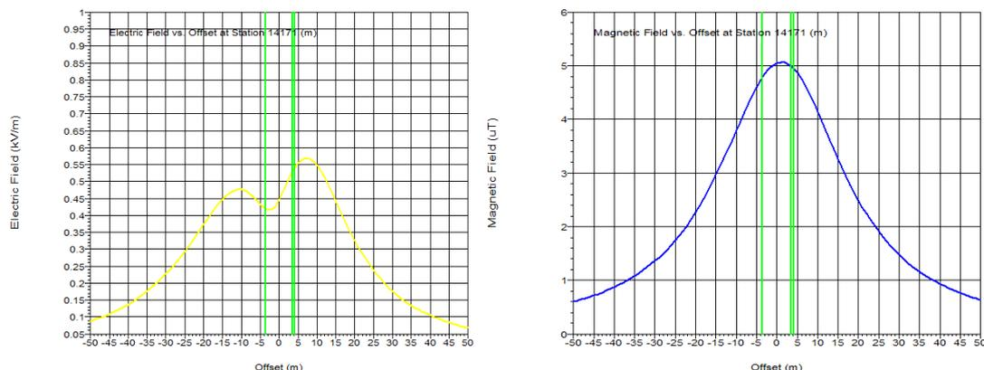
**Fig. 6:** Results of the evaluation of the electric field and magnetic field in the width of the easement strip of a 220kV transmission line with ACCC conductor. Source: [8], 2018
