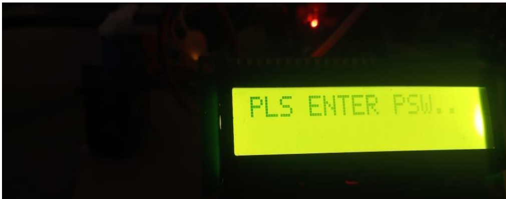
Fig 3.6: Display showing the command for entering the password.
