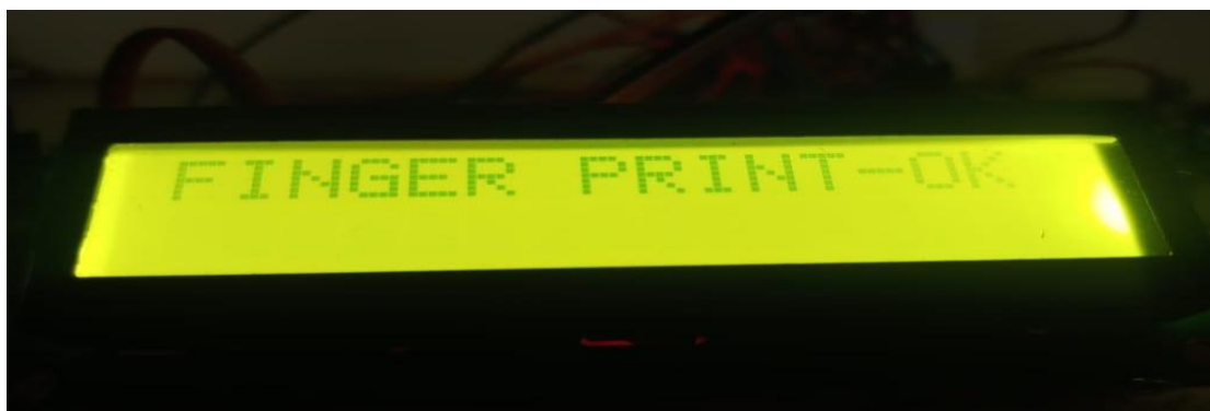
Fig 3.4: After successfully scanning the finger
