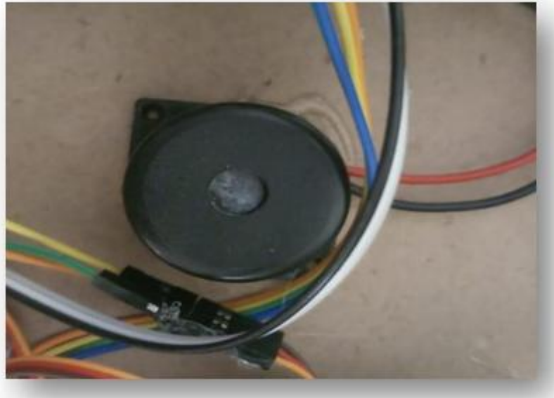
Fig 3.13: Image of the buzzer which gives a precautionary beep after entering the password for 1 st time.
