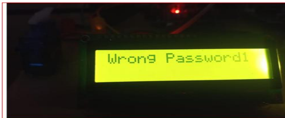
Fig 3.8: Display showing WRONG PASSWORD1 after entering the wrong password for the 1 st time.
