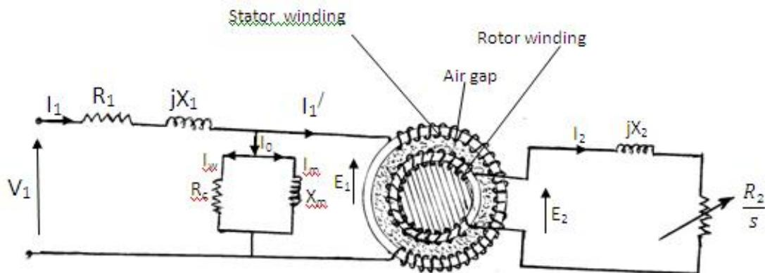
Fig. 2: Per-phase equivalent circuit of an induction motor
