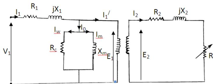
Fig 3-Per phase transformer equivalent circuit of a 3 phase induction motor with load resistance ( $R_L$ ).
