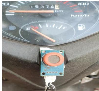
Image 3 Alcohol sensor placed on vehicle
