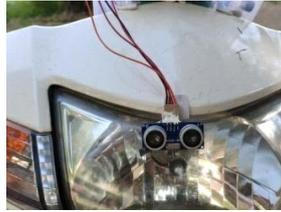
image2 Ultrasonic sensor placed on vehicle
