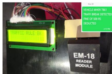
**Image 9** message display on LCD as well as Vehicle of the owner
