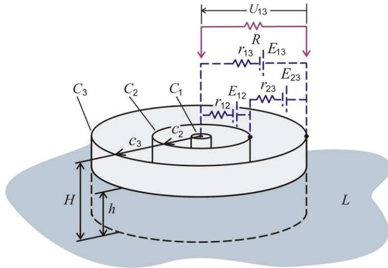
**Fig. 1.** Three cylindrical electrodes in liquid and their equivalent electromotive forces
