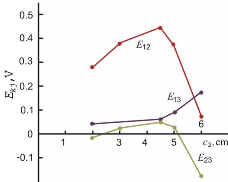
**Fig. 4.** Variations of electromotive force with radius of second electrode
