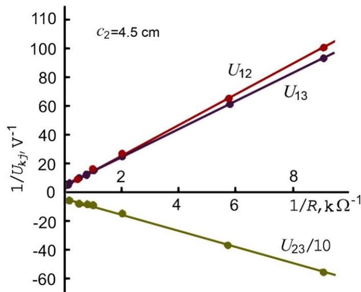
Fig. 3. Linearity of the inverse voltage versus conductivity of load resistor
