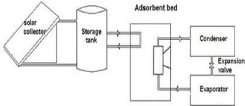
**Figure 1** Solar based adsorption refrigeration system
