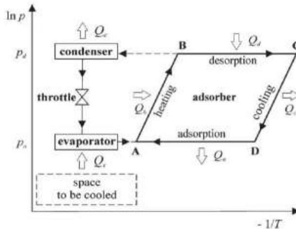
**Figure 2** Clapeyron diagram cycle for adsorption/desorption process
