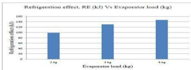
Figure 6 Variation of refrigeration effect (kJ) for different evaporator loads
