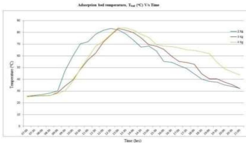
Figure 9 Adsorption bed temperature Vs Time graph
