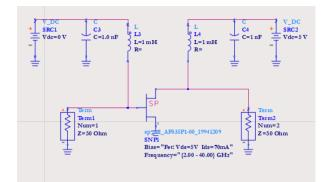
Figure 1: Schematic of the Transistor and Simulation of S parameters
