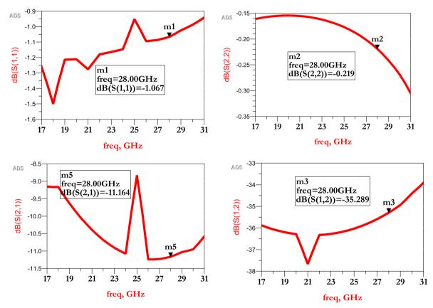
Figure 2: S parameters of the transistor
