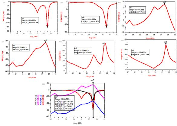
Figure 9: Parameter S of the Amplifier
