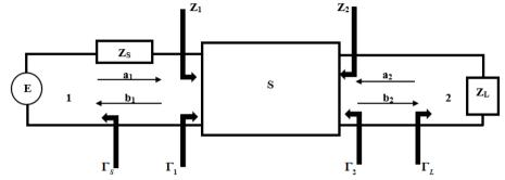
**Figure 3: Distribution waves and reflection coefficients at the entry and exit of the quadrupole** The matrix [S] of distribution of this linear quadrupole is such that <sup>9</sup>:
