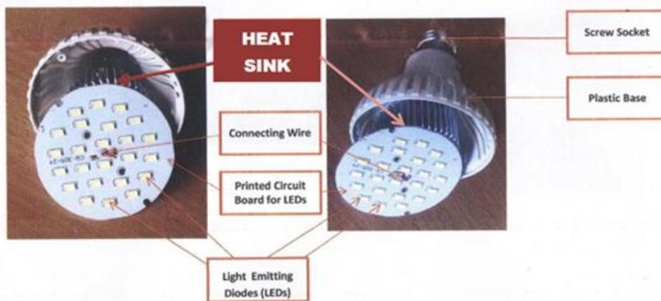
Plate 4: Novel Pin-Trapezium hybrid heat sink LED bulb
