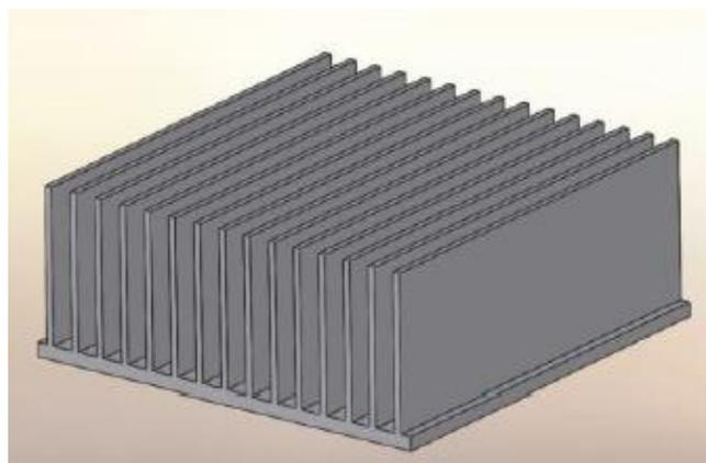
**Plate 1: Rectangular fin heat sink for LEDs**
