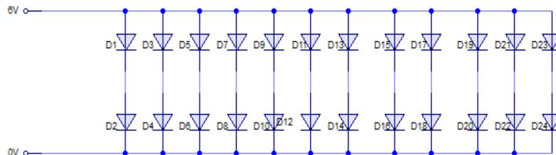
**Figure 7: LED Arrangement**
