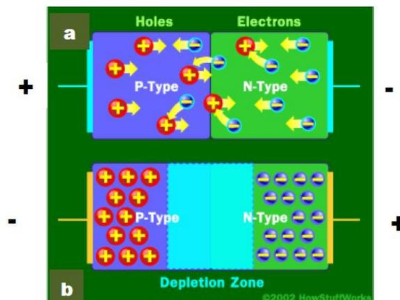
Figure 1 (a) and (b): P-N Junction
