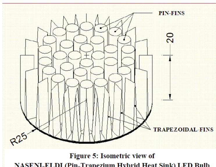
Figure 5: Isometric view of NASFNI-FI,DI (Pin-Trapezium Hybrid Heat Sink) LED Bulb
