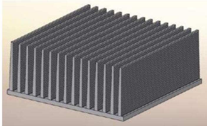
Plate 3: Trapezoidal scaled fin heat sink for LEDs
