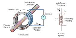
Like any other transformer, a current transformer has a primary winding, a magnetic core, and a secondary winding. The secondary winding comprises many turns of fine wire housed within the casing of the transformer.
