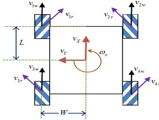
Fig 2. Kinematics of robot with Mecanum wheel
