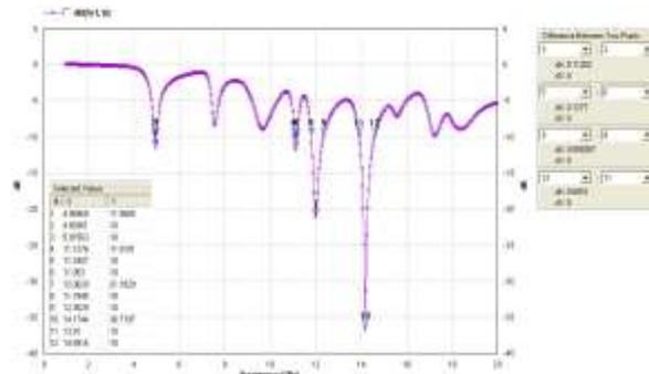
Figure 4: Return Loss vs. Frequency (Slotted Antenna)
