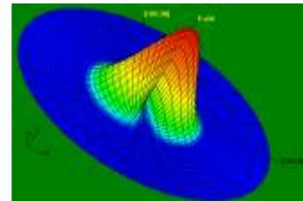
Figure 10: 3D H-Plane Radiation Pattern for Conventional Antenna at 5.46 GHz
