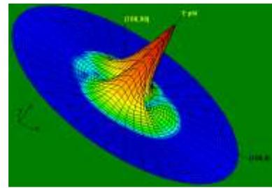
Figure 34: 3D H-Plane Radiation Pattern for slotted Antenna at 14.17 GHz
