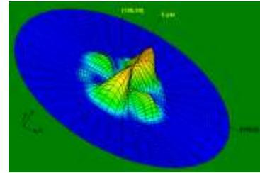
Figure 28: 3D H-Plane Radiation Pattern for slotted Antenna at 11.13 GHz
