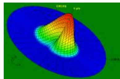
Figure 25: 3D H-Plane Radiation Pattern for slotted Antenna at 4.96 GHz
