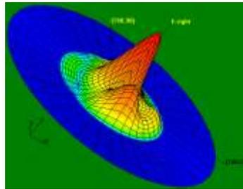
Figure 33: 3D E-Plane Radiation Pattern for Slotted Antenna at 14.17 GHz
