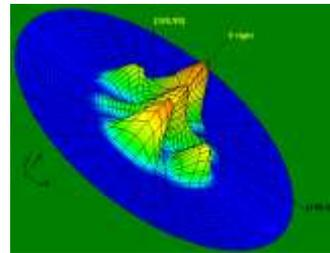
Figure 30: 3D E-Plane Radiation Pattern for Slotted Antenna at 12.00 GHz
