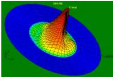
Figure 32: 3D Elevation Pattern Display at 14.17 GHz
