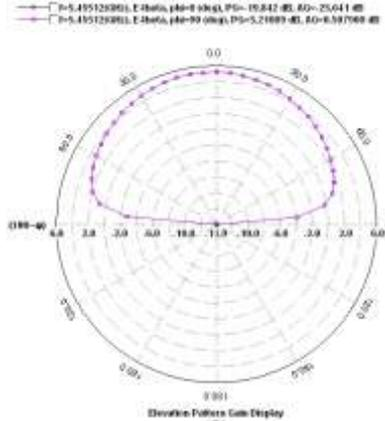
Figure 6: 2D E-Plane Radiation Pattern for Conventional Antenna at 5.46 GHz
