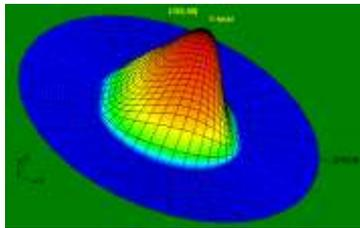
Figure 8: 3D Elevation Pattern Display for Conventional Antenna at 5.46 GHz
