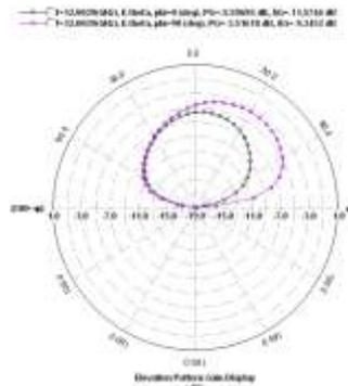
Figure 18: 2D E-Plane Radiation Pattern for Slotted Antenna at 12.00 GHz
